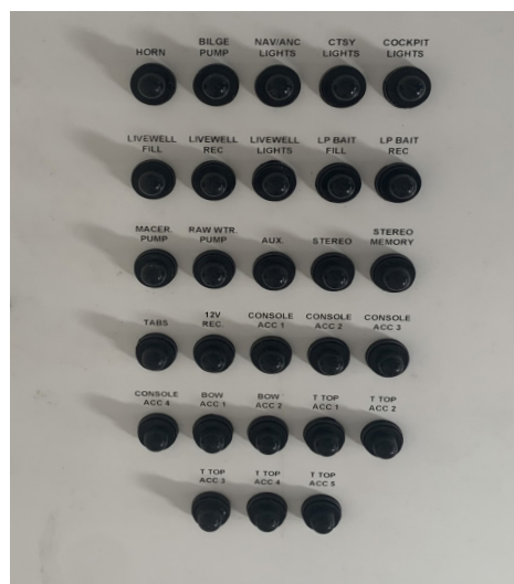
SX 2550 Breaker Panel Figure 3-13
