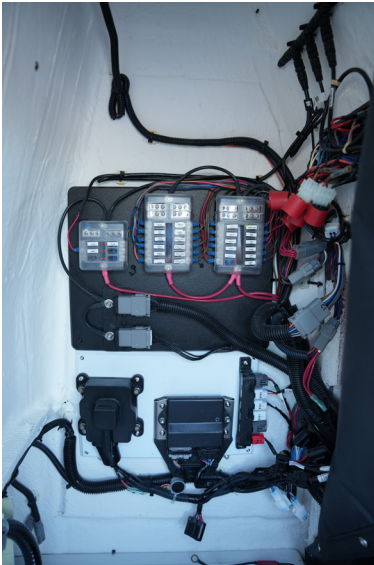
SX221, SX230, SX241, SX2350 Console Fuse panel Figure 3-12
