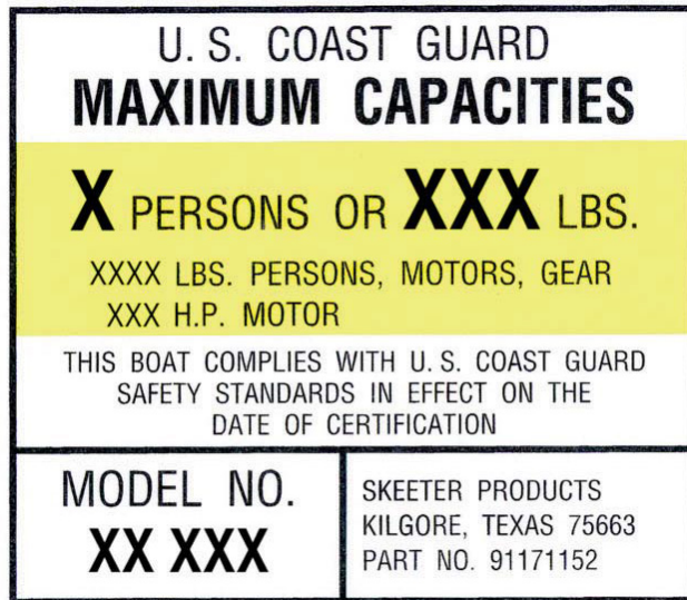
Typical Capacity Plate Figure 1-1
