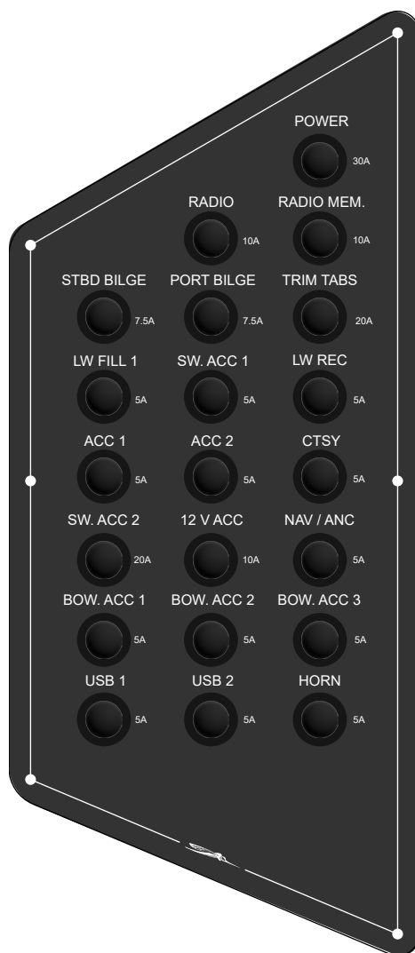
Circuit Breaker - WXR2060,WXR1910F Figure 3-13
