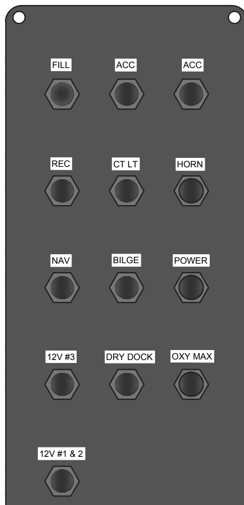
ZX Breaker Panel Figure 3-9
